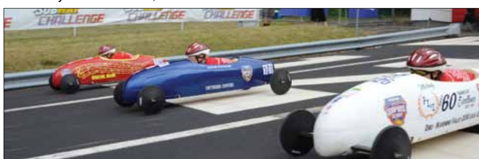
At the start of the race, Mallory (red car, far lane) is already ahead of both of her competitors. Note that her head is tucked further down and that she has a lower profile than the other drivers.
